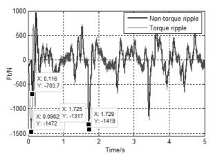
Fig. 10. Response of the dynamic load  $F_{\rm t}$  of wheel
