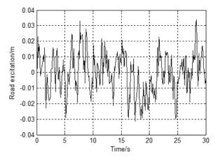
Fig. 2. The curve of Class-B Road excitation electric vehicle (speed of vehicle:  $30\,\mathrm{m/s})$
