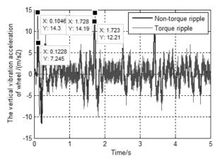
Fig. 11. Response of the vertical vibration acceleration  $\ddot{z}_1$  of wheel
