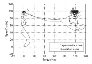
Fig. 6. Curves of motor mechanical characteristic
