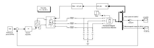
Fig. 3. Simulink model of motor
