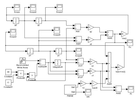
Fig. 8. The vertical vibration Simulink model of 1/4 vehicle
