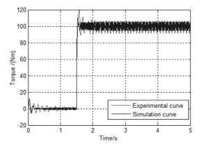
Fig. 4. Response of motor torque output
